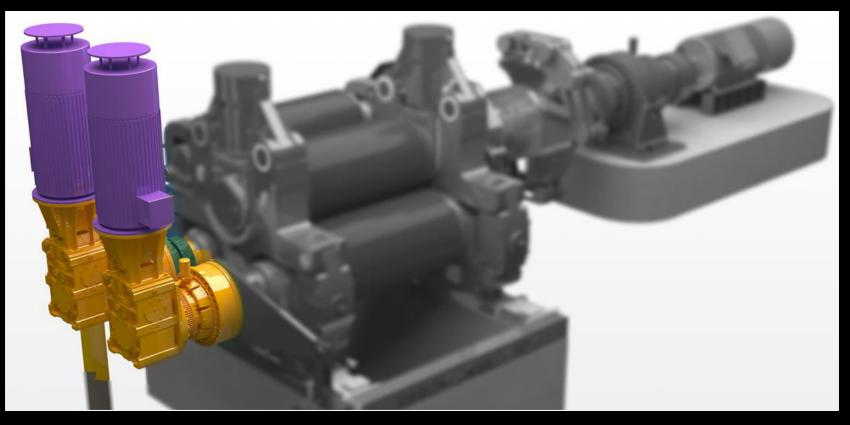
Assist drive with AC VFD to facilitate mill operations with differential roll speed.
