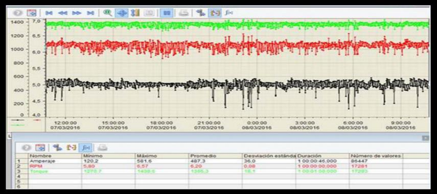
Typical DCS trend of bagasse roll of Mill no. 3
